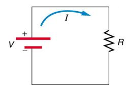
**Ohm's Law**: voltage drop = resistance (in Ohms) times current (in amps):
