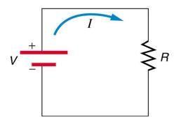
**Ohm's Law**: voltage drop = resistance (in Ohms) times current (in amps):
